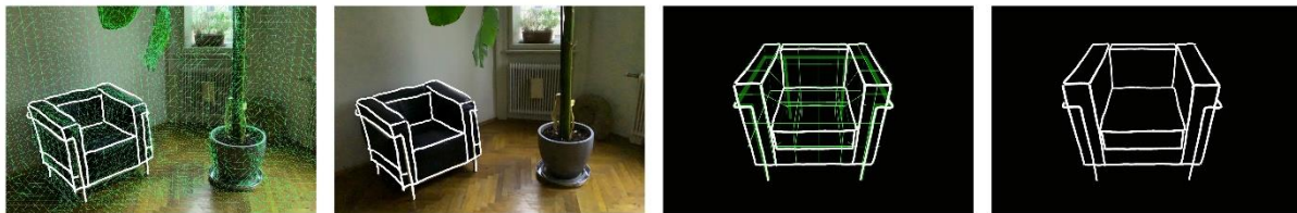
Fig. 8. Physical and virtual stocks: Using objects from stocks as drawing guides, Left: Scanning a physical seat and using it as virtual canvas, Right: Similar type of chair from the virtual stocks (Model by K. Albayrak [34])
