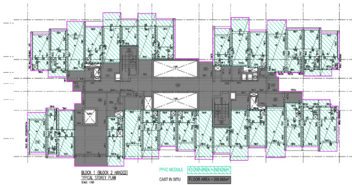
Fig. 2. Tower 1 & 2 PPVC Modularization Plan
