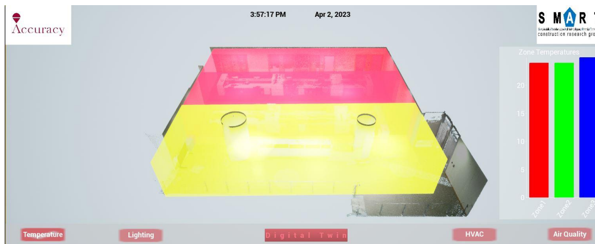
Figure 9. Screenshot of the visualization in the Unreal Engine displaying the Office Zoning Color Coding based on temperature readings from the sensors
