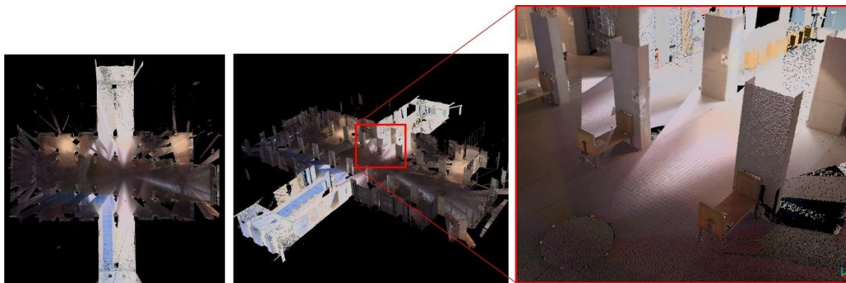
Fig. 9. Point-cloud data obtained by measuring an existing building with a 3D laser scanner.
