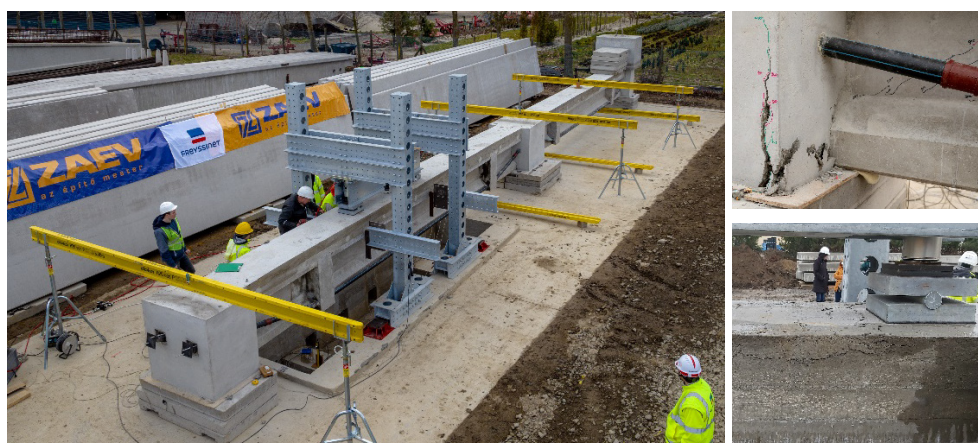
Fig. 5. Testing the “eub” type prototype structure and typical damage places at failure.
