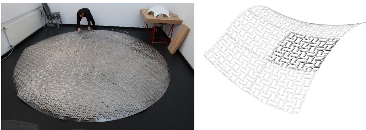
Fig. 3. Prototype 3 based on one-layer represents a pattern-coined compression-loadable membrane
