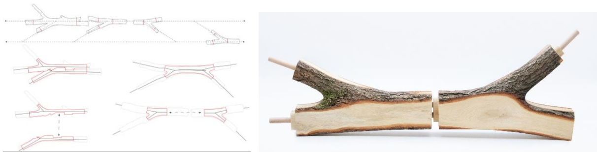
Fig. 7. Parts of a Raw-Timber-Truss with Off-Knot-Joints
