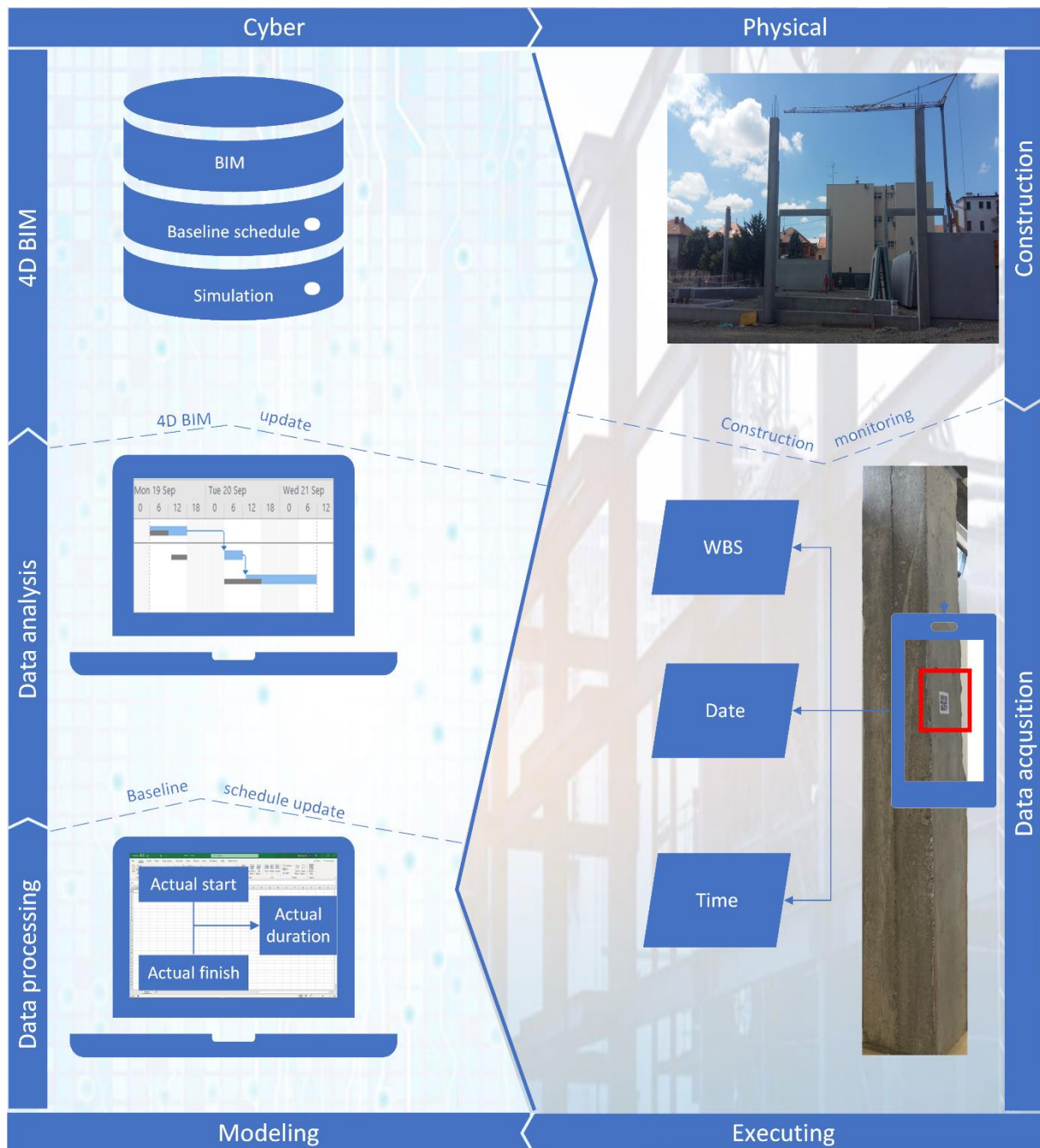
Fig. 2. Process flow of data acquisition system for automated updating of precast concrete project schedule
